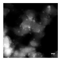
Fig.1. General scheme of selective alkyne semihydrogenation (left) and high-angle annular dark field transmission electron microscopy image of Cu nanoparticles on passivated silica (right).
