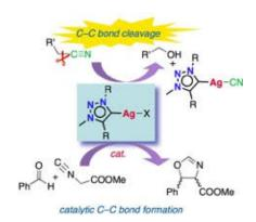
We describe that generation of Ag-NHC complexes from azolium salts in refluxing  $CH_3CN$  results in a selective C-C bond cleavage and formation of [(NHC)Ag(CN)] complexes; which can also be extended to other alkyl nitrile reagents [4].
