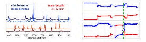
In batch distillations, finding the optimum point for the fraction change is typically the optimisation target. The short response time of Raman spectroscopy (here  $\sim$ 40 sec) allowed to reliably identify this point so that cross-contamination of the product fractions could be avoided.
