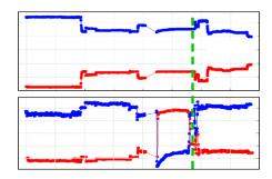
In batch distillations, finding the optimum point for the fraction change is typically the optimisation target. The short response time of Raman spectroscopy (here  $\sim$ 40 sec) allowed to reliably identify this point so that cross-contamination of the product fractions could be avoided.
