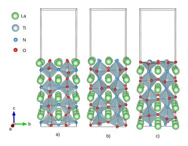
a) LaO (0.980 J/m<sup>2</sup>), b) LaN (0.542 J/m<sup>2</sup>) and c) TiO<sub>2</sub> (0.654 J/m<sup>2</sup>) terminations of the (001) surface for the energetically most preferential bulk anion order.
